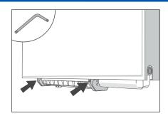
2. Turn the two locking pins outwards with an Allen key.
