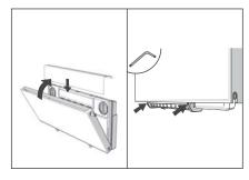
8. Install the cover and close the radiator. Then turn the two retaining pins inwards with an Allen key.
