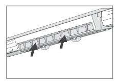
6. Press the grille at the bottom with the two clips firmly closed until you feel it snap.
