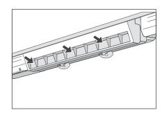
5. Place the three new filters in the sections.
