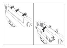
4. Open the three clips on the top and tilt the filter housing until it is open.
