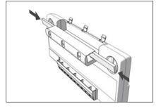
6. Slide the two new filters fully into the filter housing so that they do not project.
