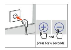
8. Push the plug back into the socket and reset the filter hour counter by simultaneously pressing on the + and - on the display for 6 seconds. The message 'Filter vervuild' will disappear.
