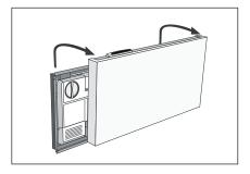
2. Remove the cover of the Sensa by lifting it upwards.
