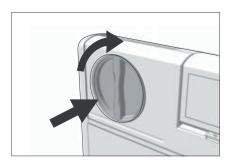
7. Install both caps and tighten them well for a correct operation.
