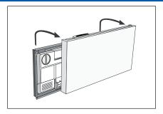
1. Remove the cover of the Sensa by lifting it upwards.
