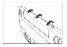
3. Open the three clips on the top and tilt the filter housing forwards.
