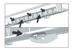
6. Push the three new filters in the sections and press the grille at the bottom with the two clips firmly closed until you feel it snap.
