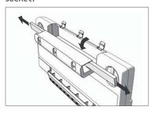
4. Slide the two contaminated filters to the sides out of the fiter housing.
