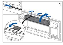
6. 1. Close the filter housing and secure with the three clips. Caution: The filters must not protrude out of the filter housing. 2. Slide the cover to the left to close.
