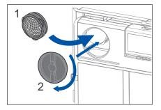
13. Insert the round cups. Install both inspection hatches and tighten them well for a correct operation.
