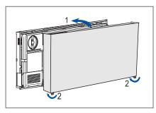
14. Put the cover back on and turn the locking hooks (at the bottom or on the side of the housing).
