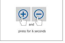
16. Reset the filter hour counter by simultaneously pressing on the + and - on the display for 6 seconds. The message 'Filter vervuild' will disappear.
