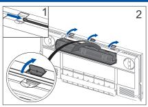
3. Replace the air supply filters. 1. Slide the cover to the right; the clips are now visible. 2. Open the three clips on the top and tilt the filter housing forwards.
