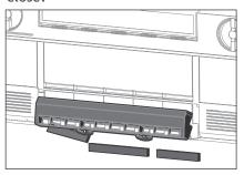
9. Push the filters from the front out of the filter housing. Place the three new filters in the sections.
