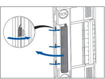
5. Close the filter housing and secure with the three clips. Caution: The filters must not protrude out of the filter housing.
