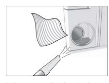
5. Remove any dirt from both channels with a vacuum cleaner or a soft cloth (do not use water).
