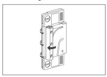
6. Tilt the filter housing back and secure with the three clips.
