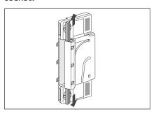
4. Push the two dirty air supply filters through the top and the bottom out of the filter housing.
