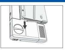
3. With a finger pull on the filter at the left-hand side of the opening and remove it.
