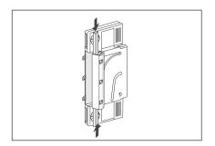
5. Push the new filters through the top and the bottom fully into the filter housing.
