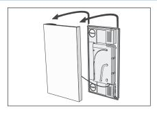
2. Remove the cover of the Sensa by lifting it upwards.
