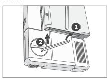
4. Insert first the right-hand side of the new filter in the outlet opening. Then push the left-hand side of the filter in the opening.
