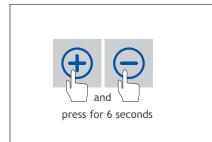
15. Reset the filter hour counter by simultaneously pressing on the + and - on the display for 6 seconds. The message 'Filter vervuild' will disappear.
