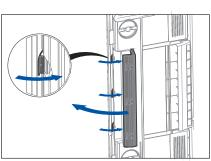
5. Close the filter housing and secure with the three clips. Caution: The filters must not protrude out of the filter housing.
