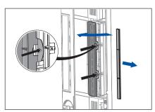
7. Replacing the air outlet filters. Unlock the filter housing by gently pulling the two clips towards you. Turn the filter grille as far forward as possible. Push the filters from the front out of the filter housing.
