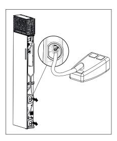
4. Remove the caps from both air ducts. Clean the duct entrances with a dry cloth or your vacuum cleaner. Also clean the insect mesh in the upper air duct. Place the caps back in the device.
