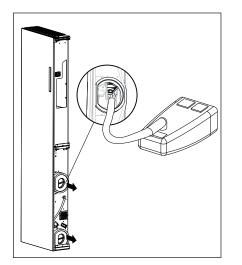
4. Remove the caps from both air ducts. Clean the duct entrances with a dry cloth or your vacuum cleaner. Also clean the insect mesh in the upper air duct. Place the caps back in the device.
