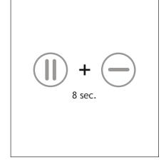
1. Set your device to service mode by holding the key combination above for 8 seconds. All LEDs will light up. Wait 1 minute for the valves to open.
