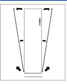
2. Remove one of the two side panels of the device.
