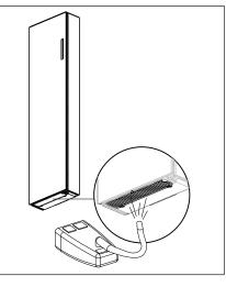
2. Clean the insect mesh at the bottom of the unit using your vacuum cleaner.
