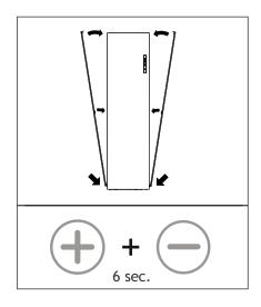
6. Place the side panel back. Reset the filter hour counter by holding the key combination above for 6 seconds. The "filter vervuild" notification will disappear.
