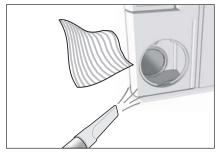
5. Remove any dirt from both channels with a vacuum cleaner or a soft cloth (do not use water).
