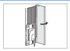
2. Open the door of the housing by lifting it up slightly on the left-hand side and then pulling it forward.
