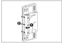
5. Tilt the filter housing back and secure with the three clips.
