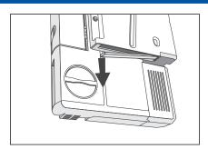
3. With a finger pull on the filter at the left-hand side of the opening and remove it.
