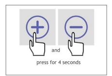
8. Reset the filter hour counter by simultaneously pressing on the + and - on the display for 4 seconds. The message 'Filter vervuild' will disappear.
