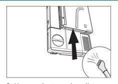
2. Vacuum the tray when dirty. You do not need to remove the air outlet filter.
