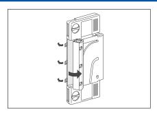
3. Open the three clips at the left-hand side of the unit and tilt the filter housing forwards
